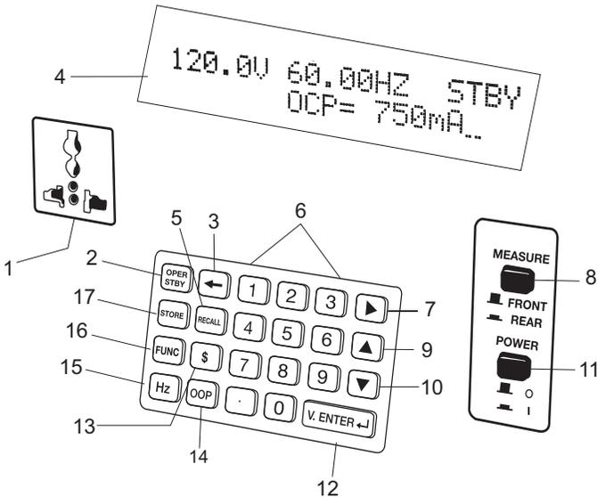
1. **Front Output Socket:** Use the following formula to determine the continuous use capability of the output:  $\text{Time (t)} = 100 / \text{Watt (w)}$ . For example, 100W power can be continuously output for 1 minute and 50W could be continuously output for 2 minutes. Switch off the tester for 20 minutes (for ventilation) between output sessions.
