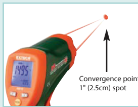
Two laser points converge at a distance of 30"/76.2cm (model 42512) or 12"/30.5cm (model 42511) and form a 1" (2.5cm) spot.
