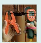
TP200 Type K clamp probe provides hands-free secure grip when measuring temperature on pipes up to 1.5" (38mm) diameter
