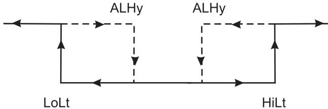
1. The alarm relay will be On when measuring value up to 100. The alarm relay will turn Off again when measuring value down to 95.
