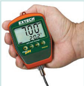
PH220-C includes pH electrode with 39" (1m) cable
