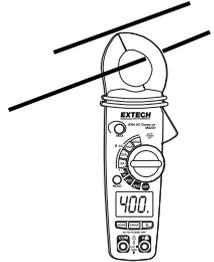
1. Set the Function switch to the **400ADC, 40ADC, 400AAC or 40AAC** range. If the range of the measured is not known, select the higher range first then move to the lower range if necessary.
