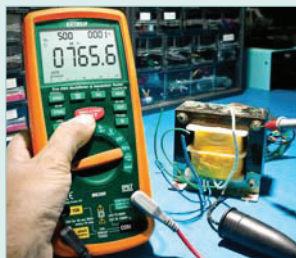
Measure the insulation resistance of transformer windings
