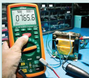
Measure the insulation resistance of transformer windings
