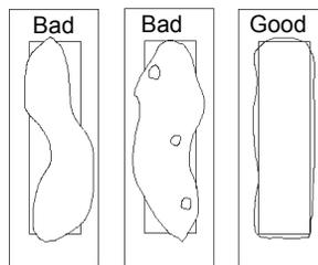
It may be necessary to adjust the position of the light source to maximize the contrast of the shadowline. Under normal conditions, optimal contrast is obtained by holding the instrument underneath and perpendicular to a light source.
