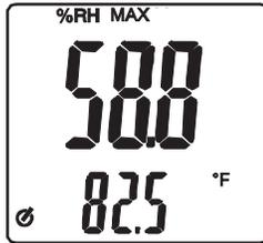
**Note:** Max and Min values are recorded into memory while the meter is on. The values are erased when power is turned off.
