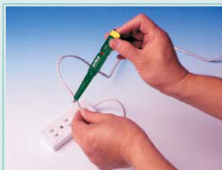
Checking for open wires in cables
