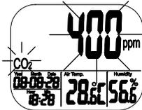
The calibration will take about 30 minutes. When the calibration is complete, the blinking stops and the meter returns to normal operation. To abort the calibration, press the **RESET** button for more than 1 second.
