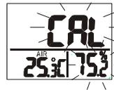
**NOTE:** Single point calibrations are allowed. To calibrate 33% only, press **CAL/Esc** and exit when 33% calibration is completed. To calibrate 75% only, press **MODE/▲** within the 5 minutes while initializing 33% calibration.
