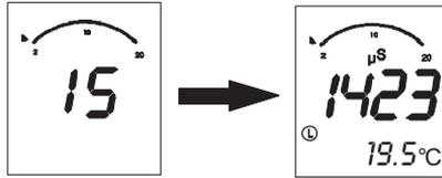
2. The last stored reading will be displayed first. Pressing and releasing the **MODE/HOLD** button will scroll through the stored readings one at a time. The location number is displayed first, followed by the reading stored in that location.
